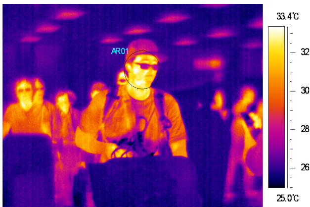
Fig. 1. The method to check the highest temperature at face by Therma CAM tm P series (FLIR Thermal Infrared Camera Systems, Inc., Boston, MA, USA)
